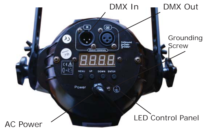
Figure 2: The Rear Connections
